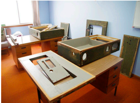
Two regulators stripped and the inside surfaces sealed
