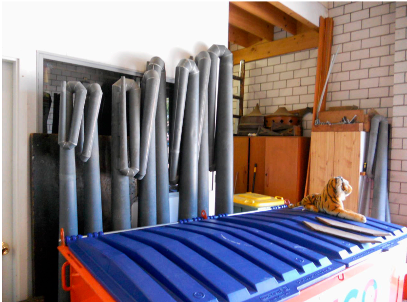
Tuba Pipes stand on end after cleaning
