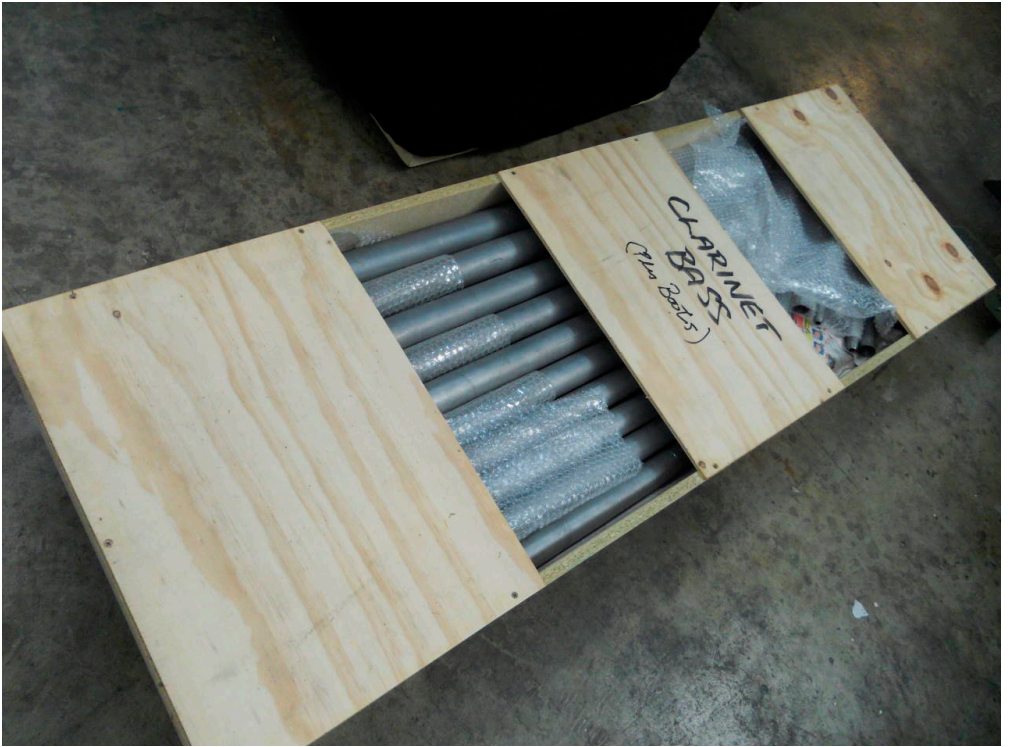
Bottom pipes of the Clarinet after cleaning plus boots
