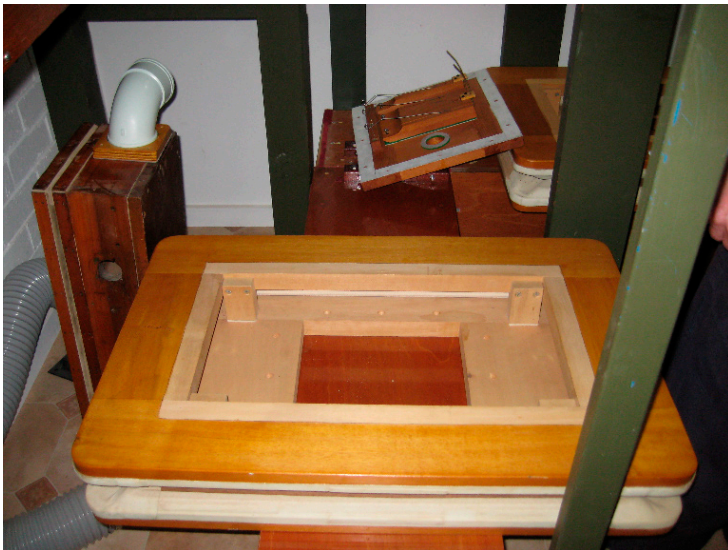
Regulator in Accompaniment chamber ready for installation
