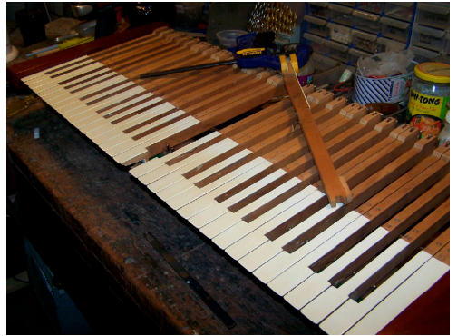
Natural keys "sides" washed, top plates reglued, celluloid playing surfaces cut and buffed.
