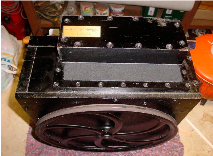
The Marrickville Wurlitzer piano pump after restoration. As you see it is a very compact unit.
