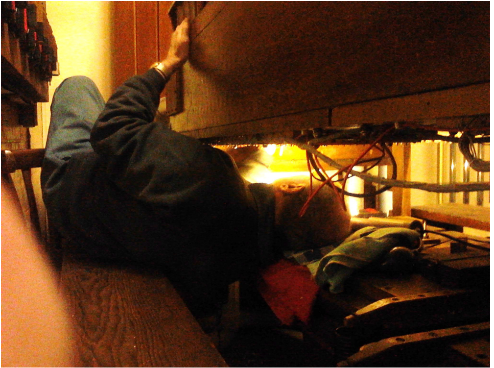
Neil Palmer balances on a walk board and regulator under the Oboe Chest whilst gluing in a secondary motor.
