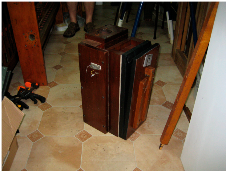
One of the completed Tremulants
