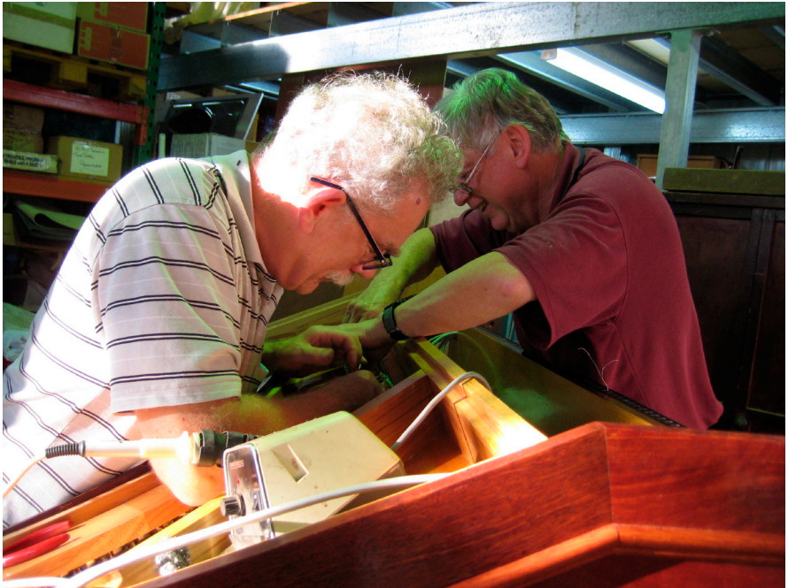
David Badman and John Weismantel connect wiring to stop rail
