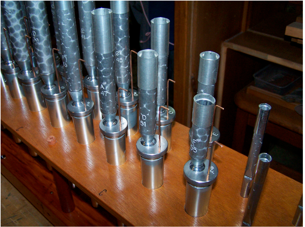
Krummet pipes in the middle of the rank as racked. Excellent presentation by organ builder John Parker
