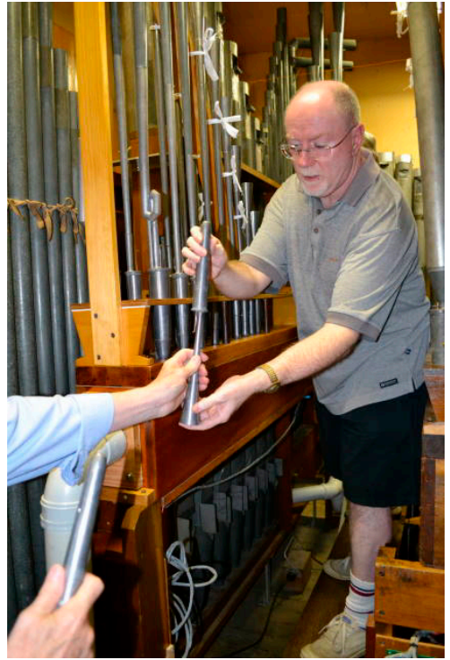
Neil Palmer takes a pipe with boot attached from John Andrews
