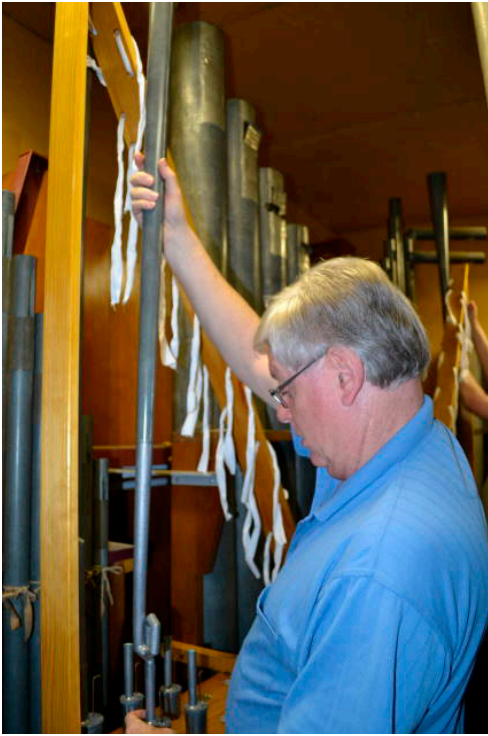
John Weismantel places a pipe into its boot already in the chest
