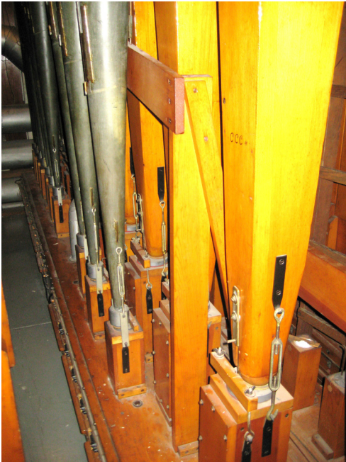
Note: both timber & metal pipes are latched to the chest so they are stable under high pressure
