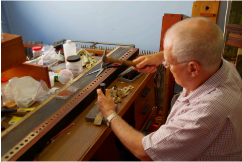
Graham Glendenning punches out a new gasket
