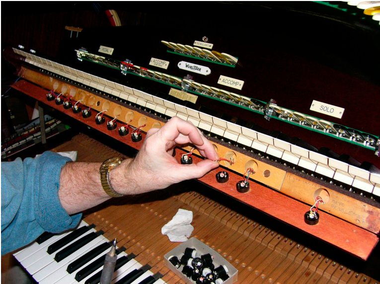
Neil Palmer works on the delicate wiring of the Piston Buttons on the Marrickville Wurlitzer
