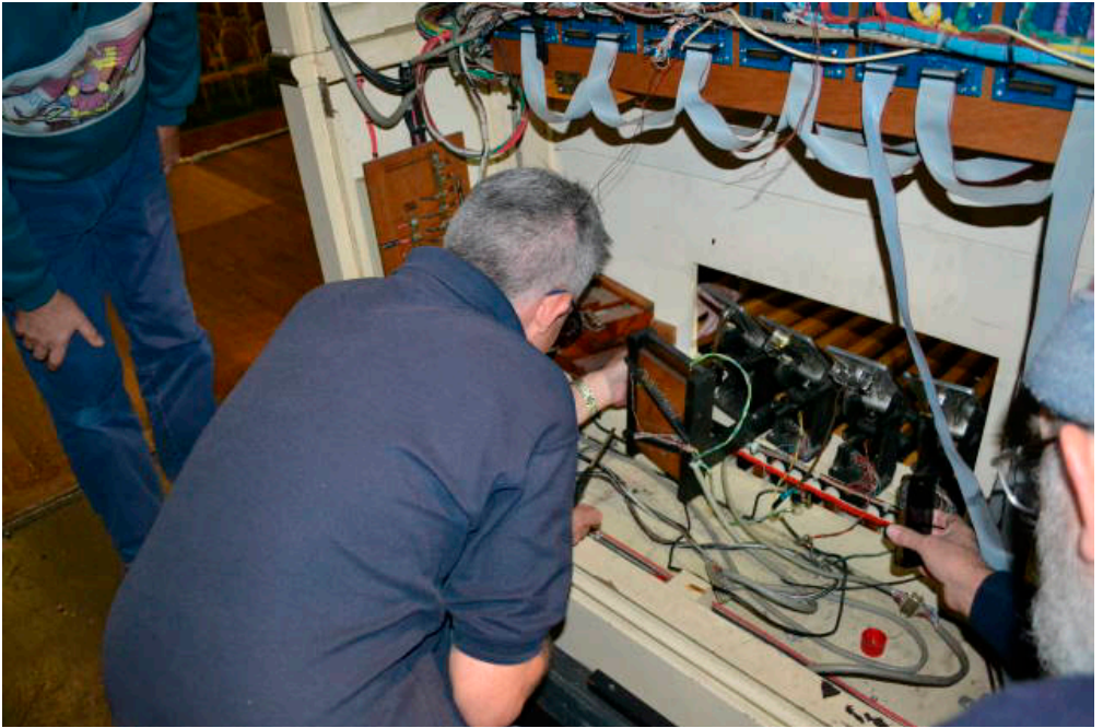
Craig Keller unscrews the block behind the four silver pedals so the pedal board can be slid away
